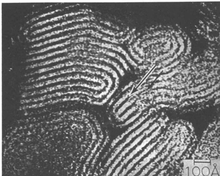
Fig. 10. Electron micrograph of lecithin micelles prepared according to FLEISCHER AND KLOUWEN 21 , negatively stained with phosphotungstate. The technique for preparing the mounts examined in the electron beam was devised by Dr. H. FERNANDEZ-MORAN, who kindly provided the photograph. The arrows point to the areas in which phosphotungstate accumulates.
